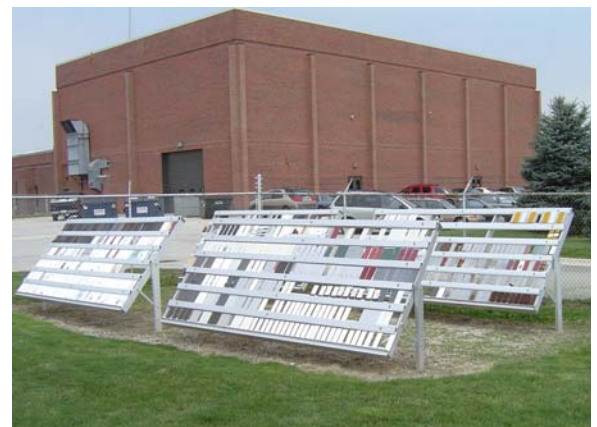
These outdoor paint-weathering racks have exposed painted metal samples to ambient environmental stresses for 10+ years.
