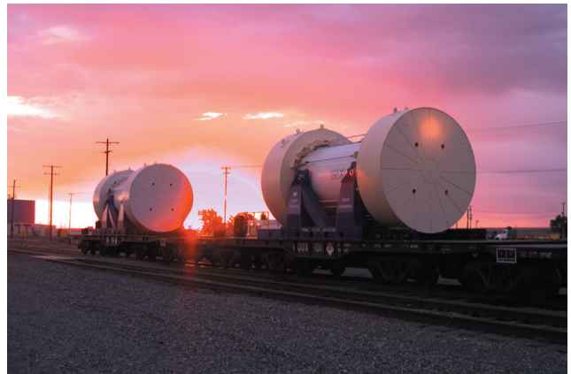
Most spent nuclear fuel and high-level radioactive waste would travel to Yucca Mountain by rail in shipping casks certified by the Nuclear Regulatory Commission.
