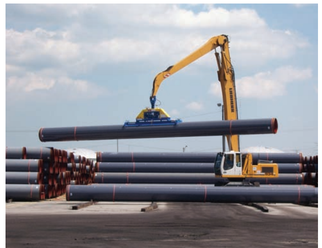
The Liebherr material handler employs a piece of vacuum equipment that simplifies and speeds up loading procedures.
