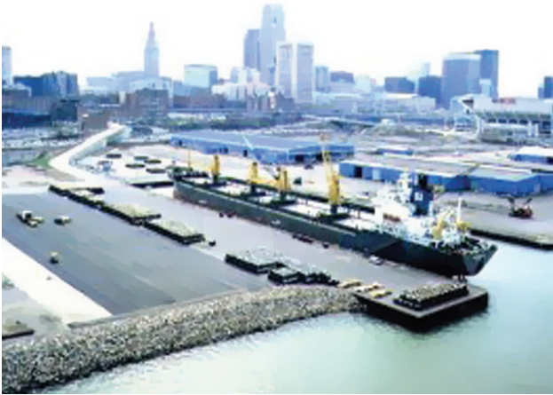
The automated CBT iron ore loader system on the west side of the Cuyahoga River loads materials onto the ships.
