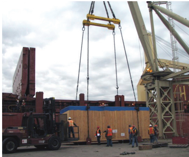
The FEDERAL POWER which came in June 2008 to the City’s heavy lift dock was unloading one of the generator parts for Algoma Energy. Cargo was transloaded to a lake barge for Algoma final destination.
