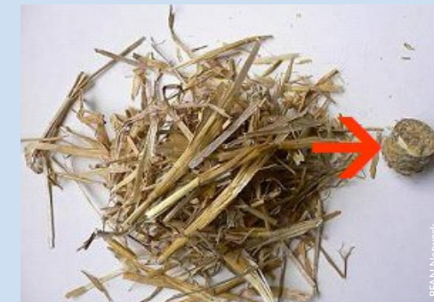
ABOVE | Biomass material converted to clean fuel pellet using densification technology
