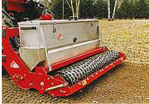
Tractor mounted seed drill
