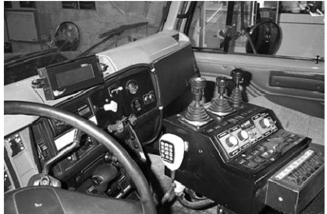
Automated Vehicle Location (AVL) unit.
