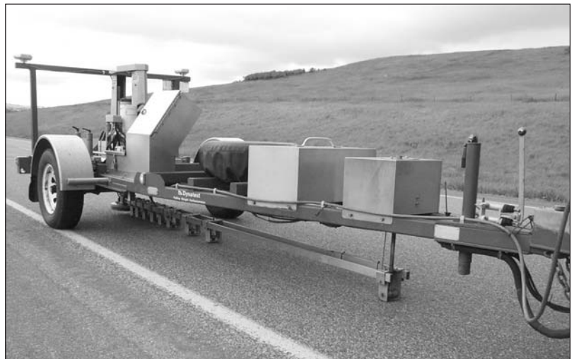
This falling weight deflectometer is used to test pavement condition.
