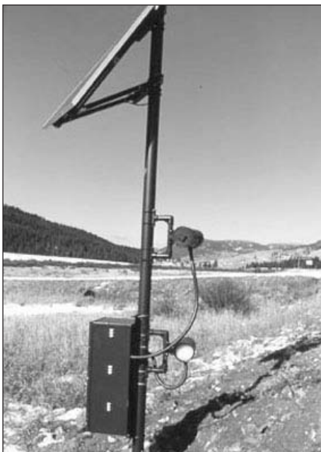
This series of photos shows an animal-vehicle crash mitigation system that is the subject of current pooled-fund study.
