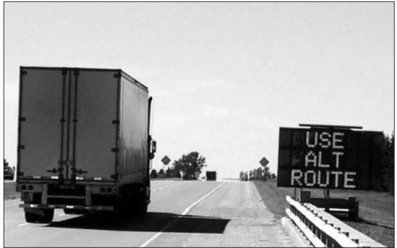
Dynamic message signs are one example of ITS technology.
