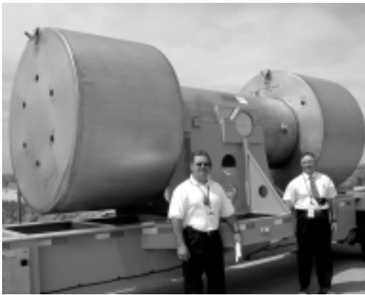
RH-72B cask at the WIPP. This cask will be used to ship remote-handled TRU waste to WIPP for disposal.
