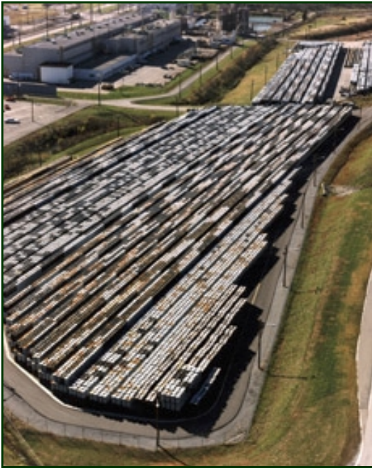
Oak Ridge—Outside drums used to store sludge containing both hazardous and radioactive waste. Over a period of time the drums rusted and have since been packed in special plastic containers and stored indoors (see picture below).
