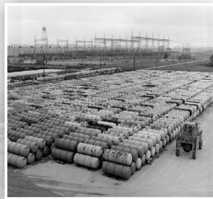
Storage yard of depleted uranium hexafluoride cylinders
