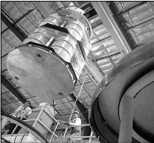
A group of 14 drums of transuranic waste at INEEL being lowered into a Trupact-2 shipping cask
