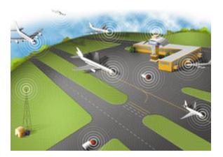
ADS-B-equipped aircraft broadcast their precise position, speed, and altitude via a digital datalink. ADS-B receivers that are integrated into the air traffic control system or installed aboard other aircraft provide users with an accurate depiction of real-time aviation traffic, both in the air and on the ground.
