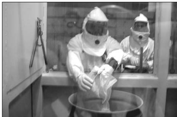
Workers begin treating the first radioactive sludge retrieved from a loadout pit.
