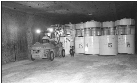
Waste handling technicians emplacing transuranic waste at a Department site.
