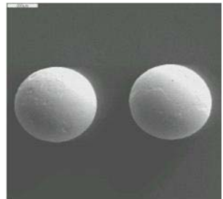
Uranium carbide particles produced by atomization at INL.
