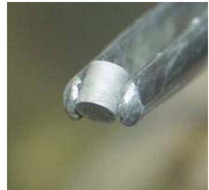
Low-fertile AFC-1G nitride fuel pellet fabricated at LANL.
