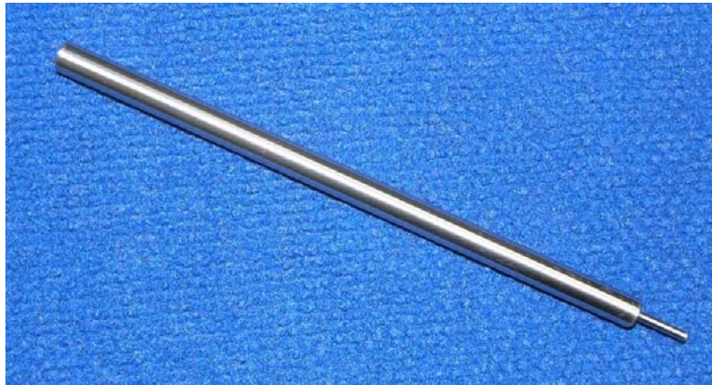
Surrogate sphere-pac pin fabricated at ORNL
