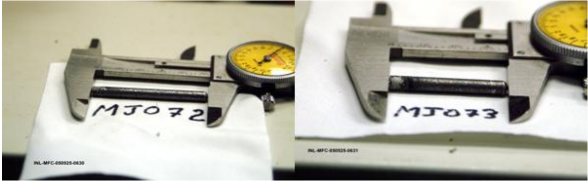
Un-sectioned pieces of the U-29Pu-2Np-4Am-30Zr metal alloy FUTURIX-FTA fuels fabricated by arc-casting.
