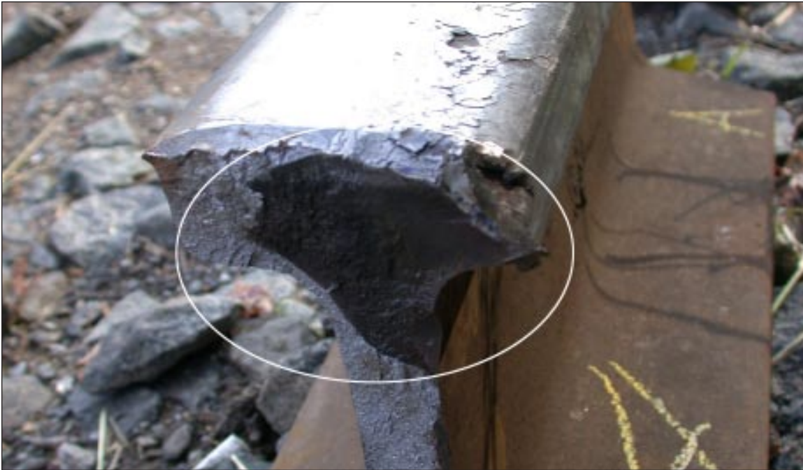
Figure 3. Recovered rail showing detail fracture from shelling in head area.
