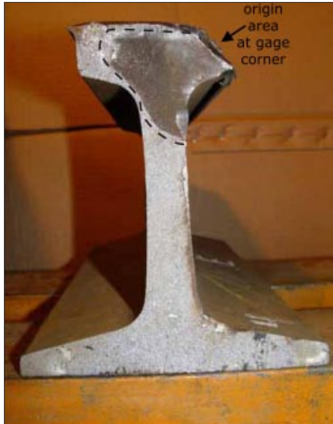
Figure 6. View of east surface of fracture 4. (The dashed line indicates the boundary of a detail fracture covering about 78 percent of the worn rail head and extending into the web. The defect emanated from an open shell crack at the gage corner.)
