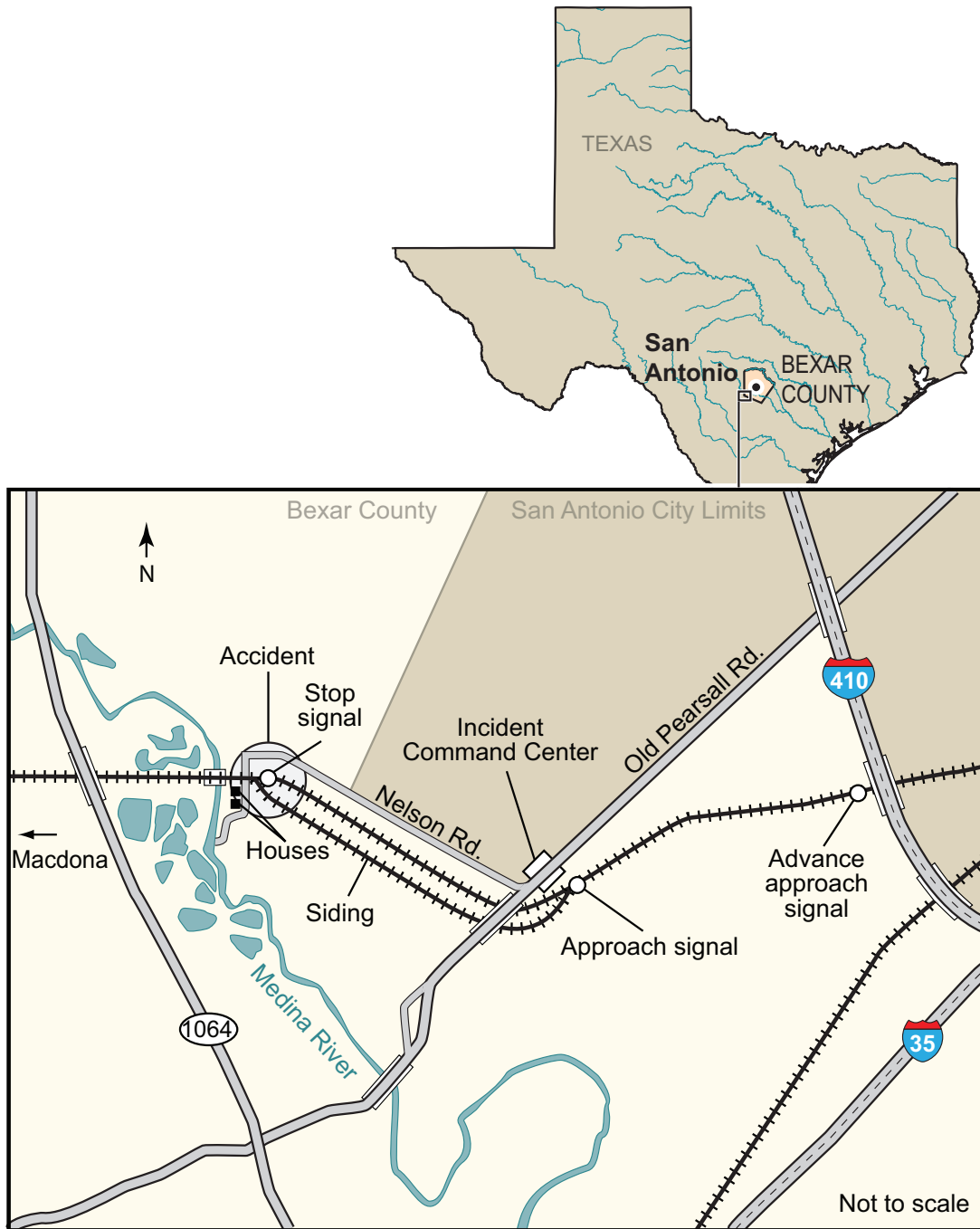
Figure 2. Portion of Union Pacific Railroad main line between San Antonio, Texas, and accident site at Macdona. Signals are identified with indications displayed for accident Union Pacific Railroad train.
