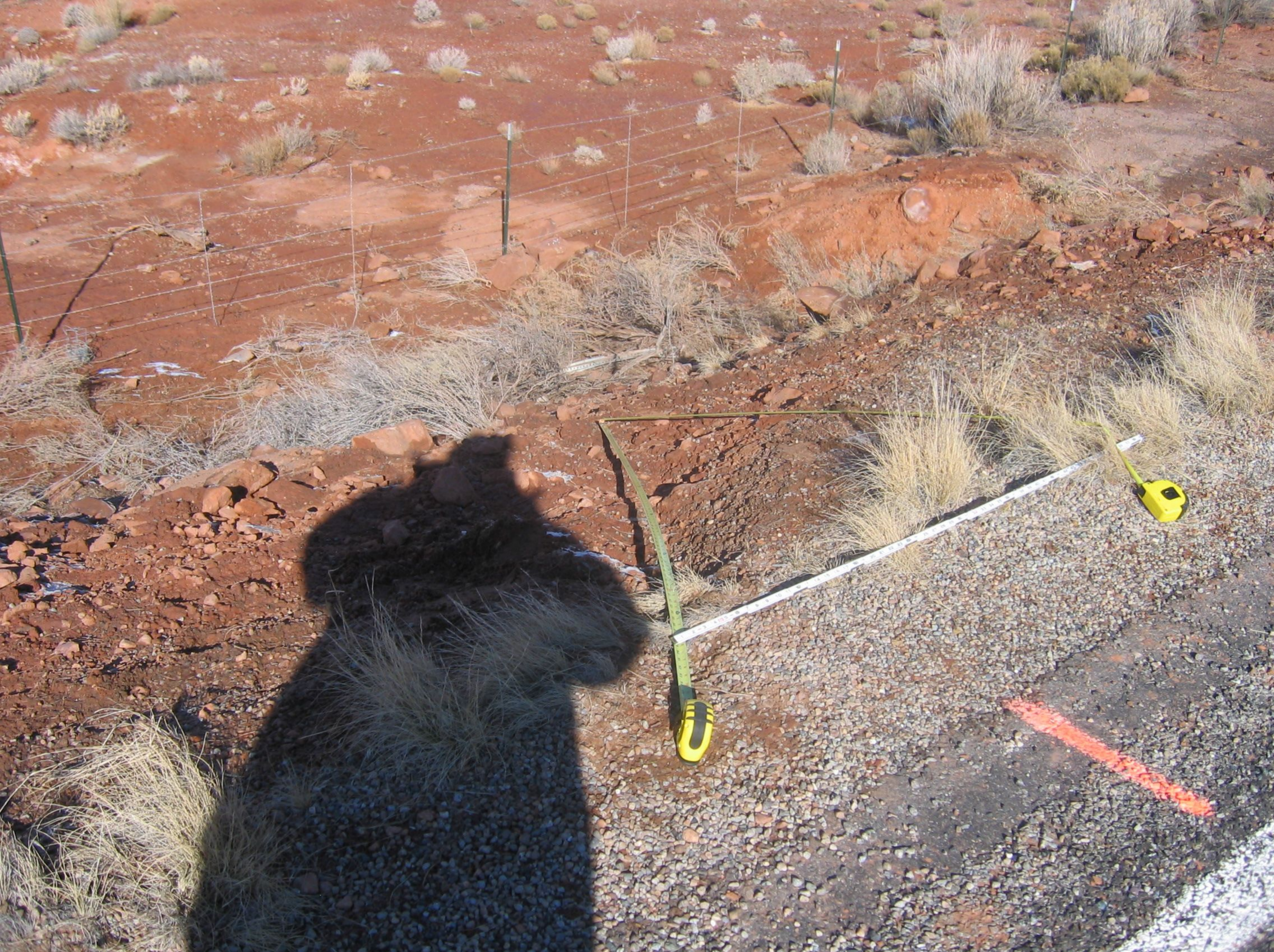
Hwy. Photo #26 - View of ground scar indicating the bus was oriented at approximately 37 degrees to the roadway
