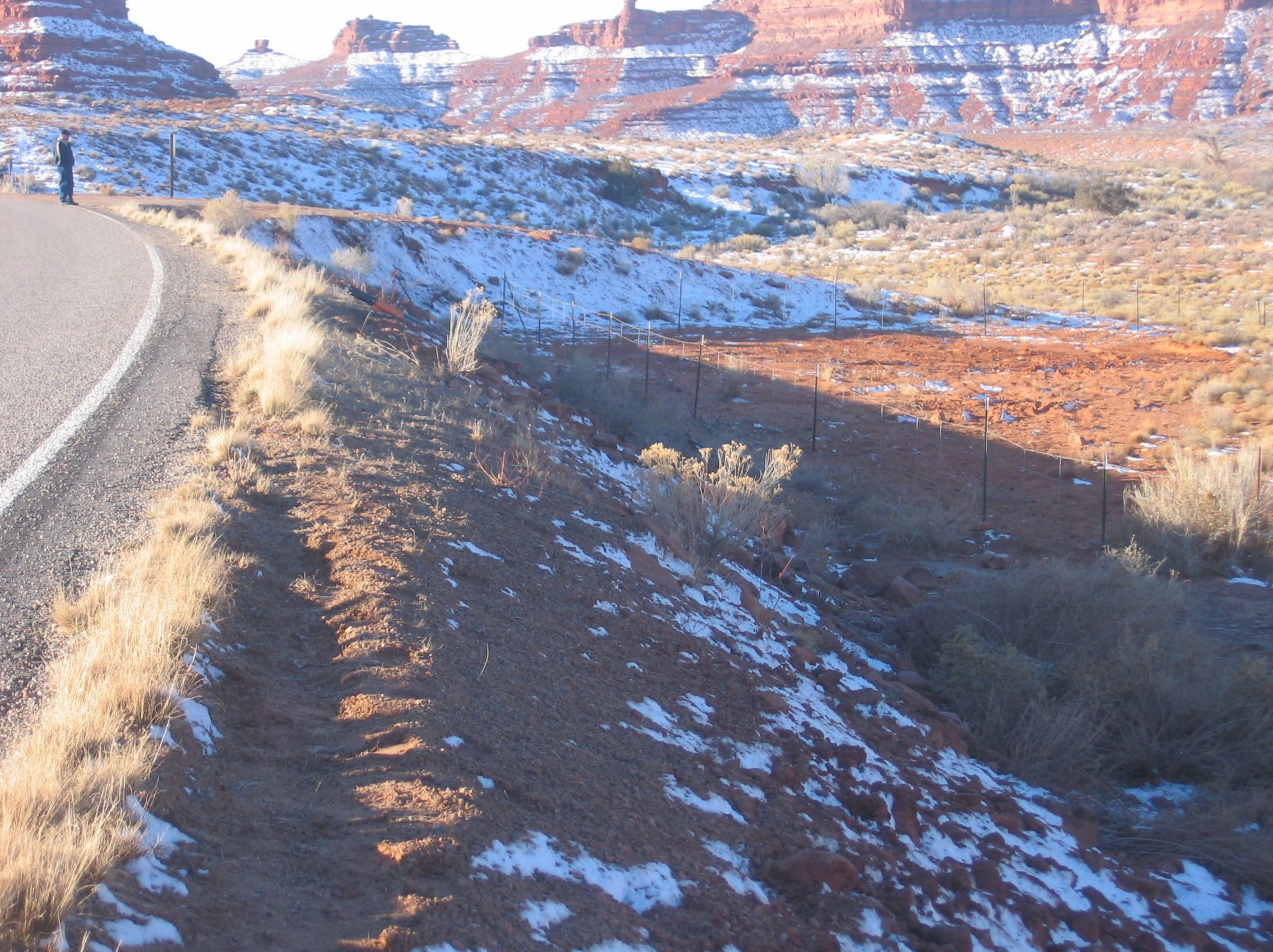
Hwy. Photo #17 - Note the furrowing of the motorcoaches' left front tire as it curves back toward the white painted edge line.
