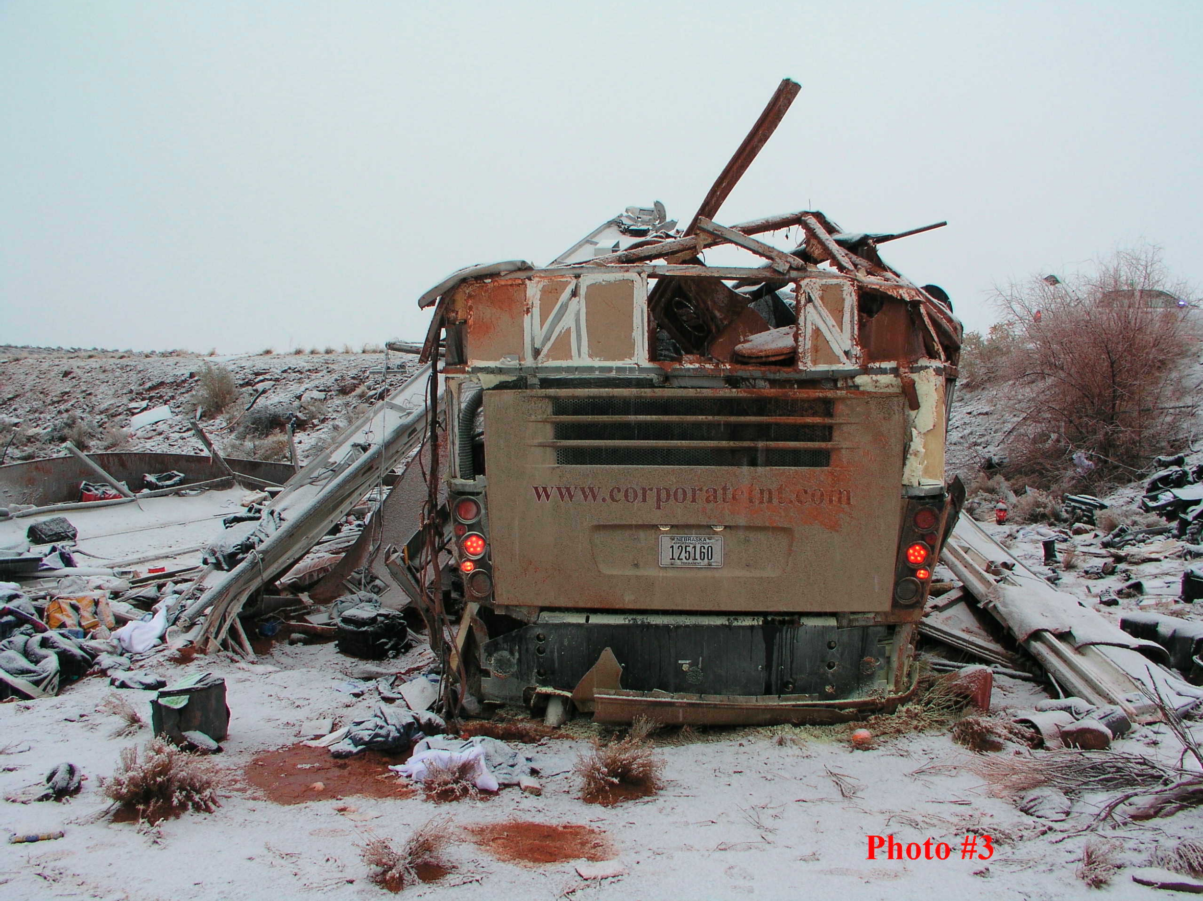
Veh. Photo #03 - Rear of MCI bus in final resting position (Note rear brake lights illuminated)
