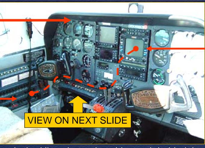
The dashed line shows the wiring path behind the instrument panel of a similar airplane
