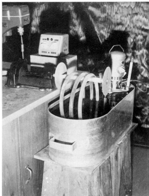
FIGURE 3. Equipment for rotating tubing filled with milk or cleaning solution.
