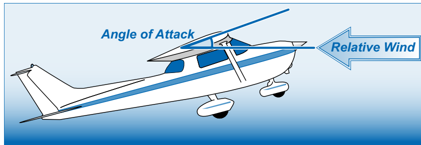
Angle of attack between oncoming relative wind and aircraft wing centerline.
