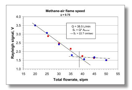
The laser-based Rayleigh scattering technique was selected to determine flame speed. Studies are under way to verify this technique using a flat-flame burner in our laboratory applied to the methane-air system. Flame speed measurements for the methane-air flame are abundant in the literature, so this provides a means to characterize the expected experimental uncertainties for this measurement technique.
