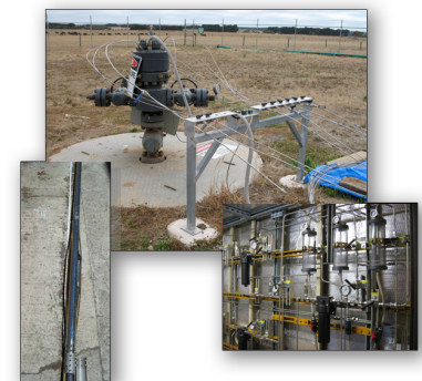
Otway Naylor-1 monitoring well completed (top) with seismic (l), geochemical (r), and other reservoir monitoring instrumentation.
