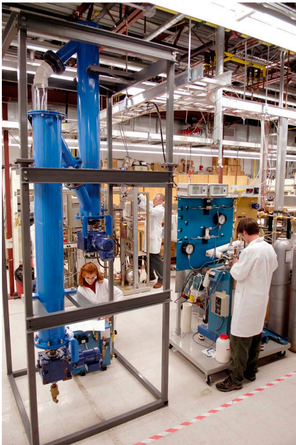
Figure 2. The lab-scale demonstration unit of RTI's dry-carbonate process
