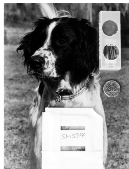
Figure 2. Photograph displaying simulated placement of retrospective detectors on picture-frame glass. The retrospective surface monitor is located toward the bottom of the glass surface and the retrospective reconstruction detector is located in the top right-hand corner of the glass surface. Coin is provided to indicate scale.
