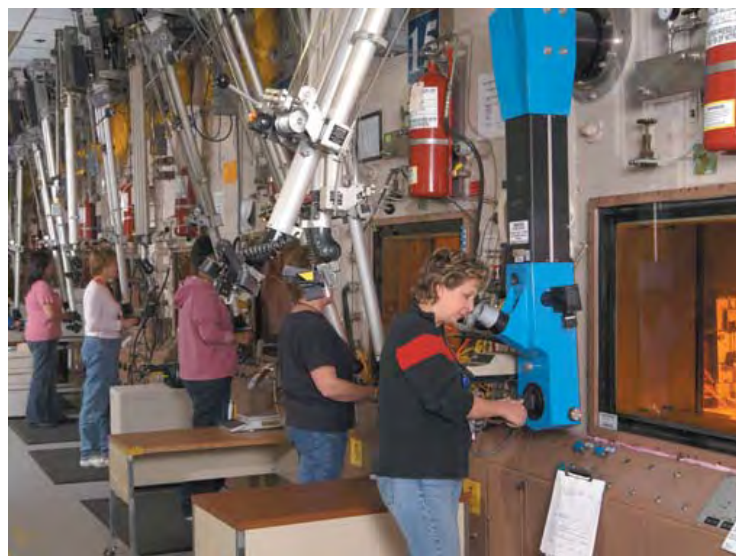
In addition to the manipulators, the shielded cells include equipment for a variety of analytical and research tasks
