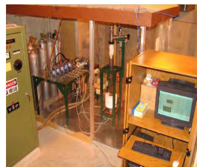
Fluidized bed, chemical vapor deposition system for advanced coated particle fuel development
