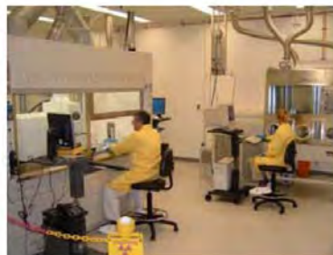
Radiochemistry laboratories provide chemical fume hoods and glove boxes for specialized analyses.
