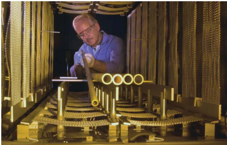
A DOE laboratory researcher holds a metal-supported ceramic membrane. The thin membranes are applied to the inner surface of the tubular supports. These membranes are used for the separation and purification of hydrogen.
