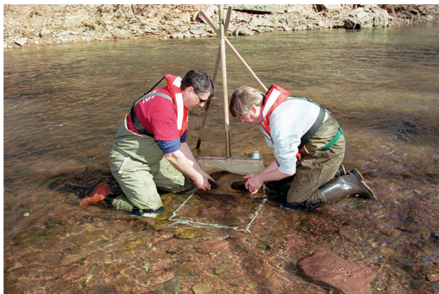
Figure 6. Slack sampler with 425-micron mesh being used for Richest Targeted Habitat (RTH) sampling in New Jersey (Photograph by Denis Sun, U.S. Geological Survey)
