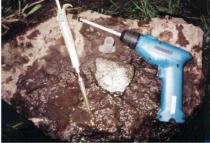
Figure 7. Algal sampling equipment used in New Jersey streams including (from left to right) a pipette, the cut-off barrel portion of a 30-milliliter syringe above a flat rock with three circular algal samples removed, and a hand-held cordless drill with a brush bit.
