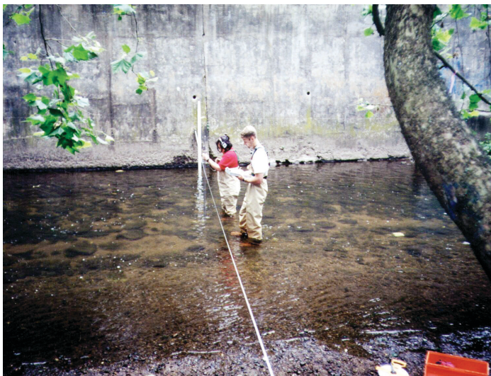
Figure 4. Water velocity being measured along one of six transects at Saddle River at Ridgewood, N.J. (01390500).
