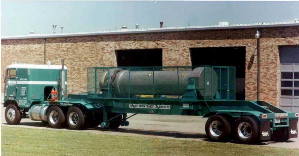
Figure 4.5. NAC LWT Transport Package (without ISO container)
