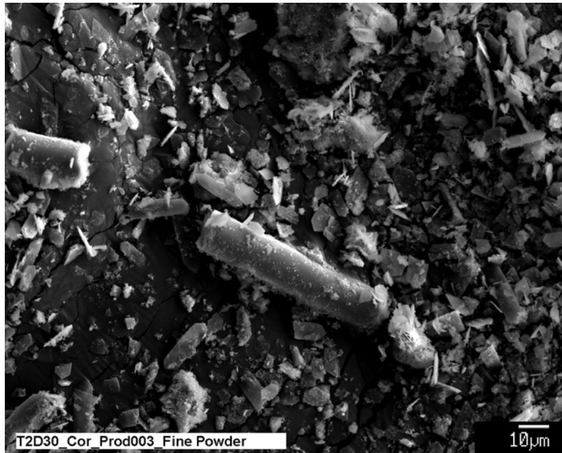
Figure B-4. Another SEM image at 650 \times magnification for a Test #2, Day-30 sample of fine powder on a vertical piece of the submerged PVC rack. The cylinder-shaped debris is likely to be fiberglass. (T2D30_Cor_Prod003_Fine Powder)
