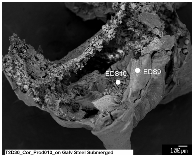
Figure B-17. Backscatter SEM image at 55× magnification for a Test #2, Day-30 sample of corrosion products on a submerged GS coupon, annotated to show EDS sample locations. (T2D30_Cor_Prod010_on Galv Steel Submerged)
