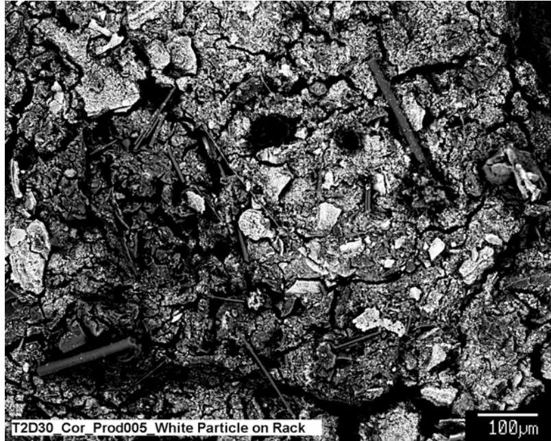
Figure B-7. Backscattered SEM image at 130× magnification for a Test #2, Day-30 sample of white residue on a horizontal piece of the submerged PVC rack. (T2D30_Cor_Prod005_White Particle on Rack)
