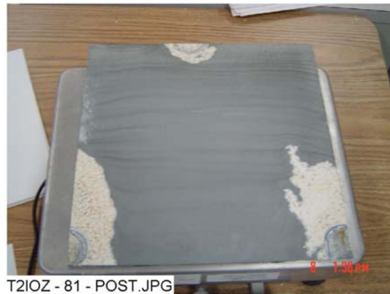
Figure 4-17. IOZ-81 submerged, post-test.
