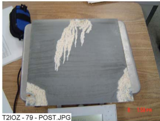
Figure 4-15. IOZ-79 submerged, post-test.
