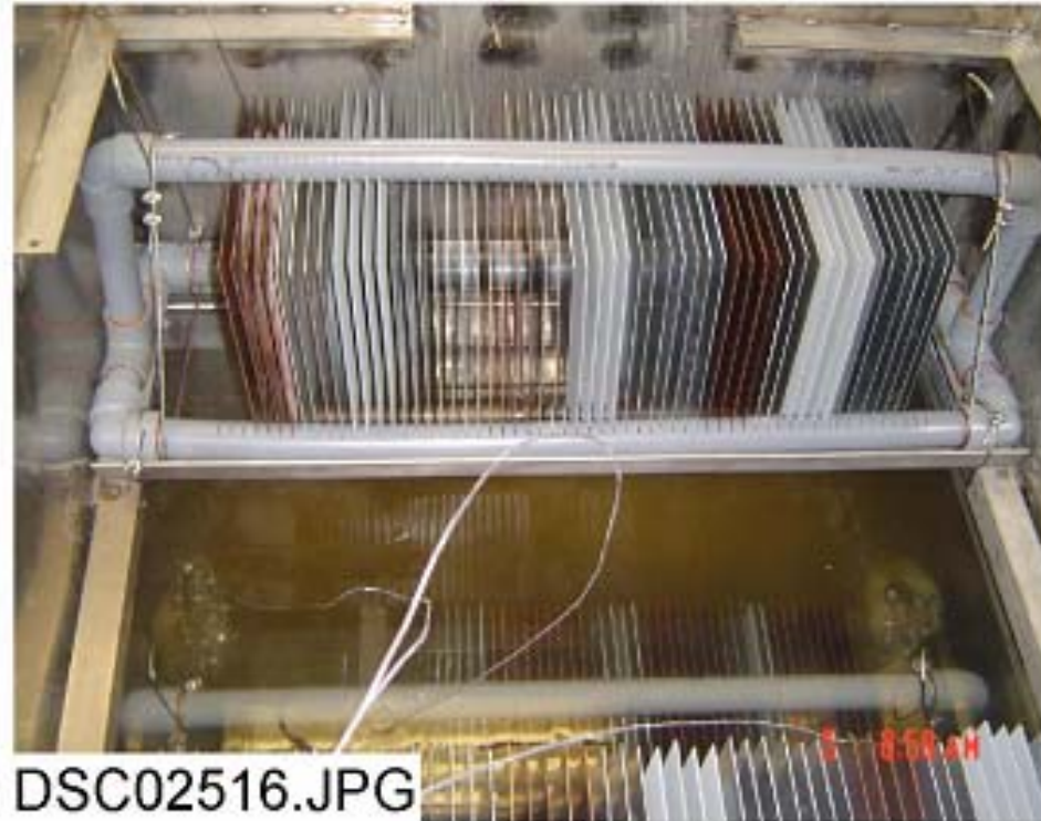
Figure 3-3. Loaded coupon rack in the ICET tank.
