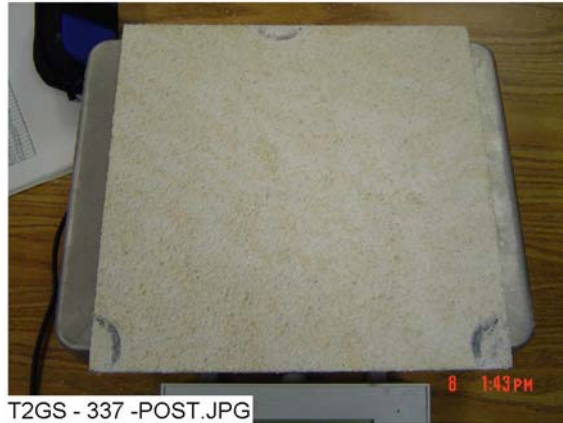
Figure 4-11. GS-337 submerged, post-test.
