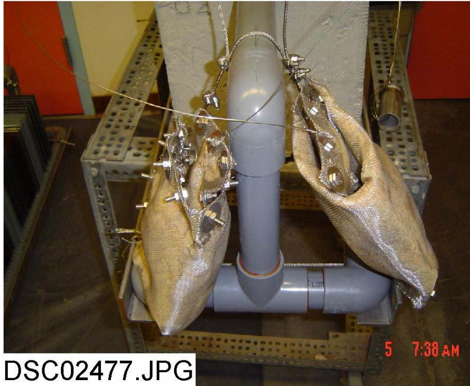
Figure 3-4. Fiberglass samples attached to the submerged coupon rack.
