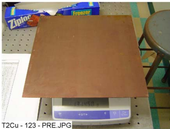
Figure 4-20. Cu-123 submerged, pre-test.
