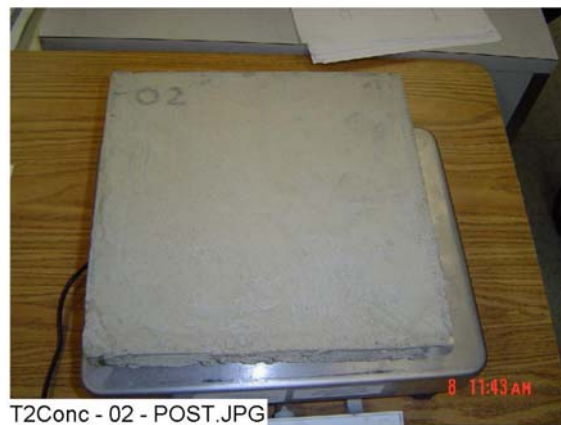
Figure 4-25. Conc-02 submerged, post-test.
