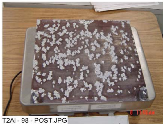
Figure 4-7. Al-98 submerged, post-test.
