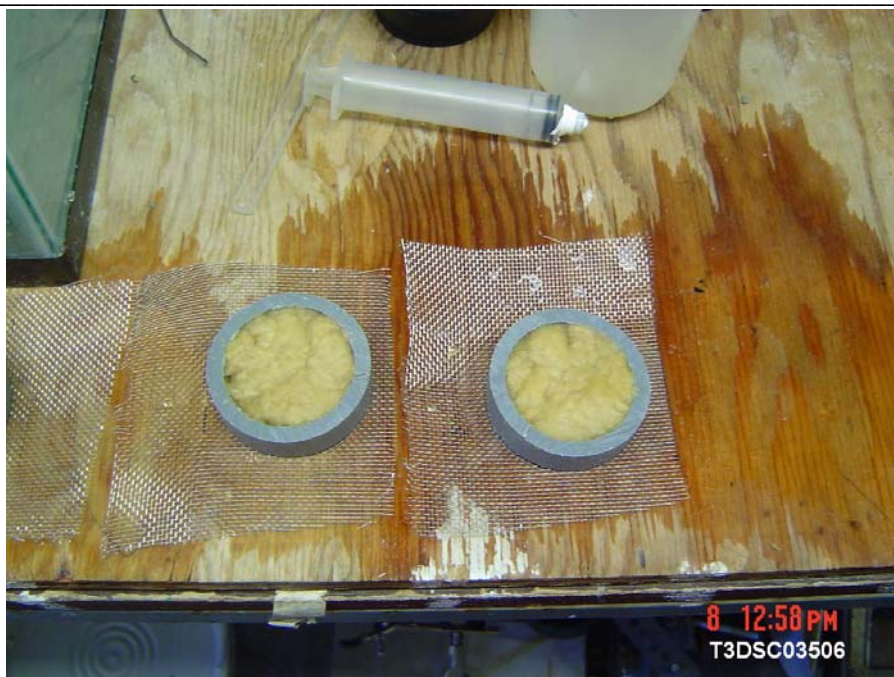
Figure 1. Example fiber pucks prepared for immersion in ICET test solution.
