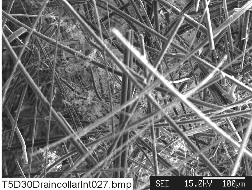
Figure C6-13. Probe SEM image magnified 200 times for a Test #5, Day-30 interior drain collar fiberglass sample. (T5D30DraincollarInt027.bmp)
