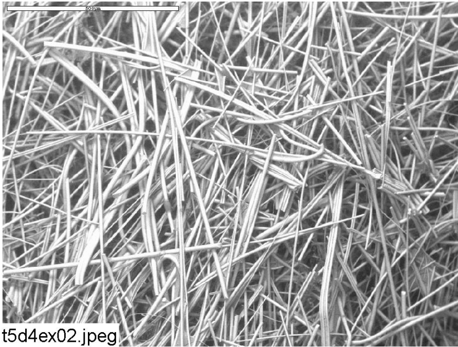
Figure A-2. ESEM image magnified 100 times for a Test #5, Day-4 low-flow exterior fiberglass sample. (t5d4ex02.jpeg)
