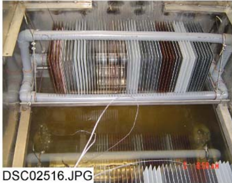
Figure 2-3. A typical loaded coupon rack in the ICET tank.
