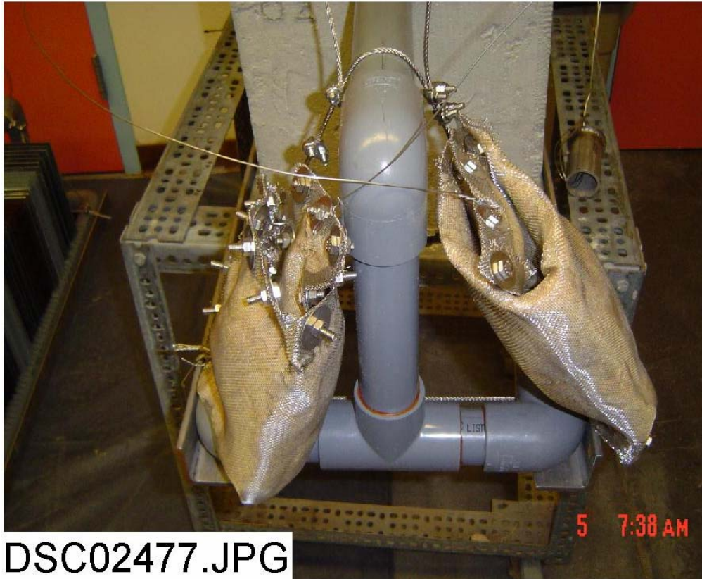
Figure 2-4. Fiberglass samples attached to a coupon rack.
