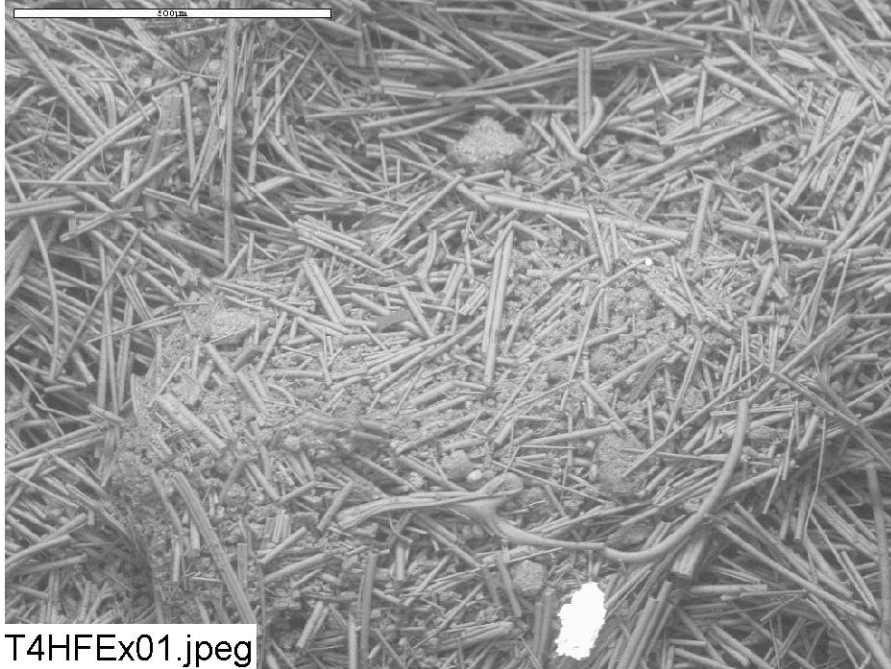
Figure C4-1. Environmental SEM image magnified 100 times for a Test #4, Day-30 exterior high-flow fiberglass sample. (T4HFEx01.jpg)
