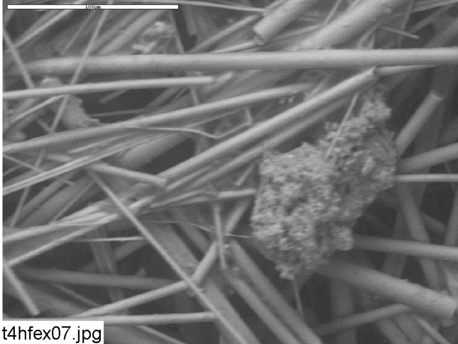
Figure C4-3. Environmental SEM image magnified 500 times for a Test #4, Day-30 exterior high-flow fiberglass sample. (t4hfex07.jpg)
