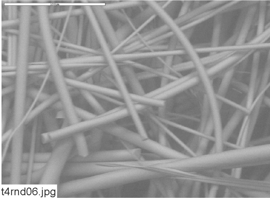
Figure C4-15. Environmental SEM image magnified 500 times for a Test #4, Day-30 interior high-flow fiberglass sample. The sample was gently prerinsed with RO water. (t4rnd06.jpg)
