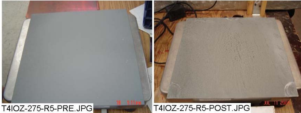
Figure 3-117. IOZ-275 unsubmerged, pre-test (left) and post-test (right).
