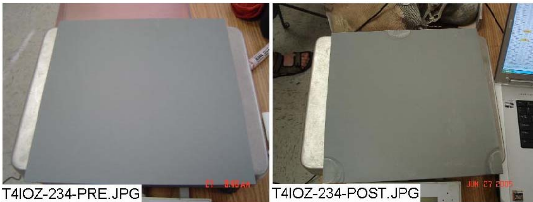
Figure 3-105. IOZ-234 submerged, pre-test (left) and post-test (right).
