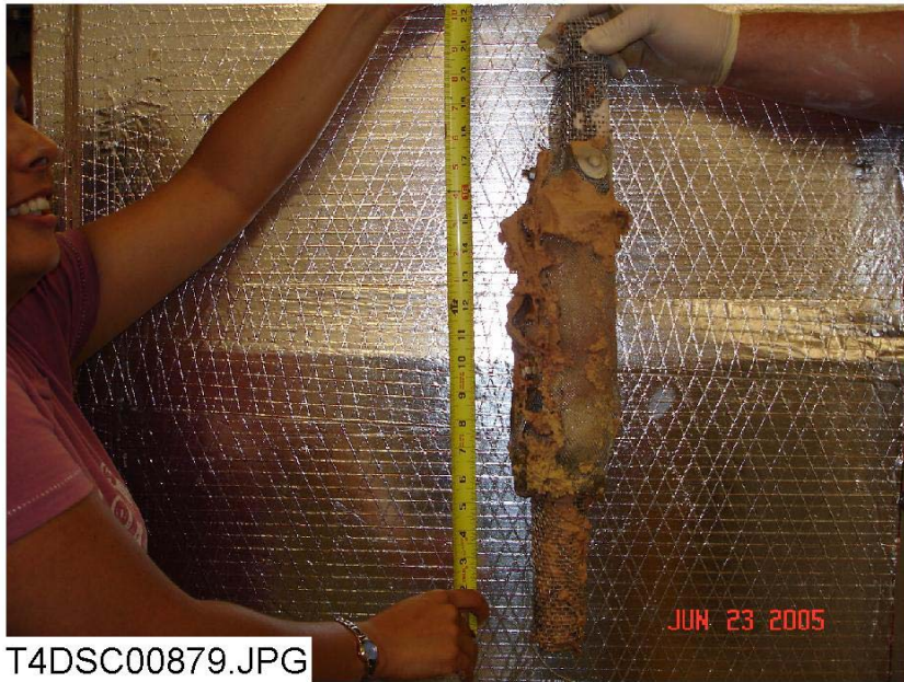
Figure 3-122. Drain collar and drain screen removed from the tank.
