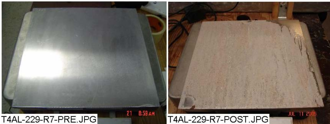
Figure 3-111. Al-229 unsubmerged, pre-test (left) and post-test (right).
