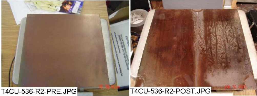
Figure 3-114. Cu-536 unsubmerged, pre-test (left) and post-test (right).
