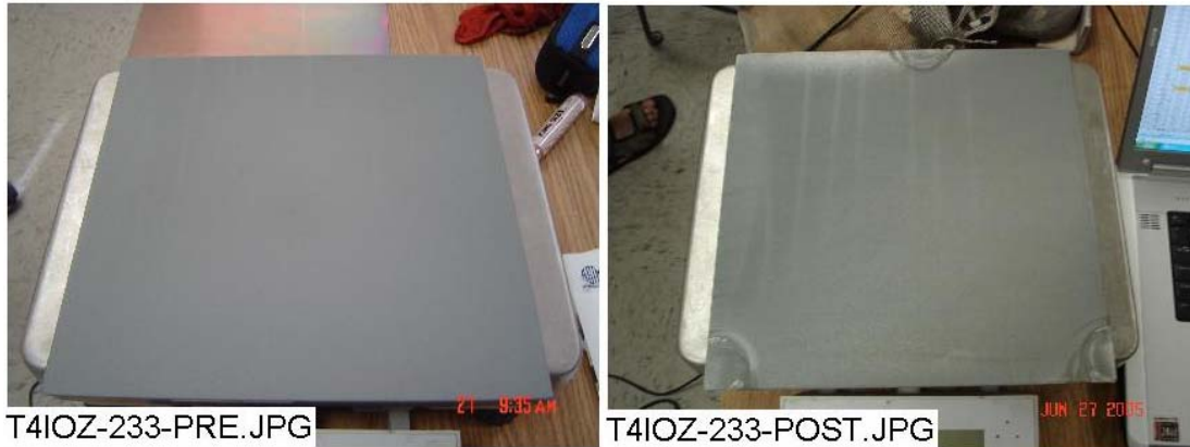
Figure 3-104. IOZ-233 submerged, pre-test (left) and post-test (right).
