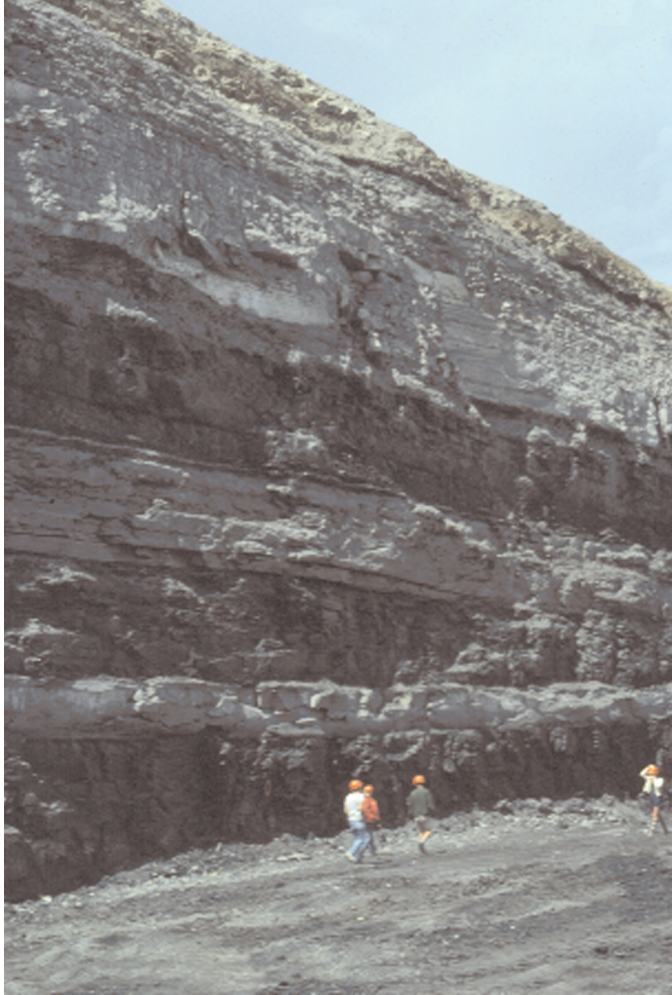
Figure 30. Working face in Kayenta mine, Black Mesa, Arizona exposing three 10-ft-thick coal beds in the Wepo Formation.
