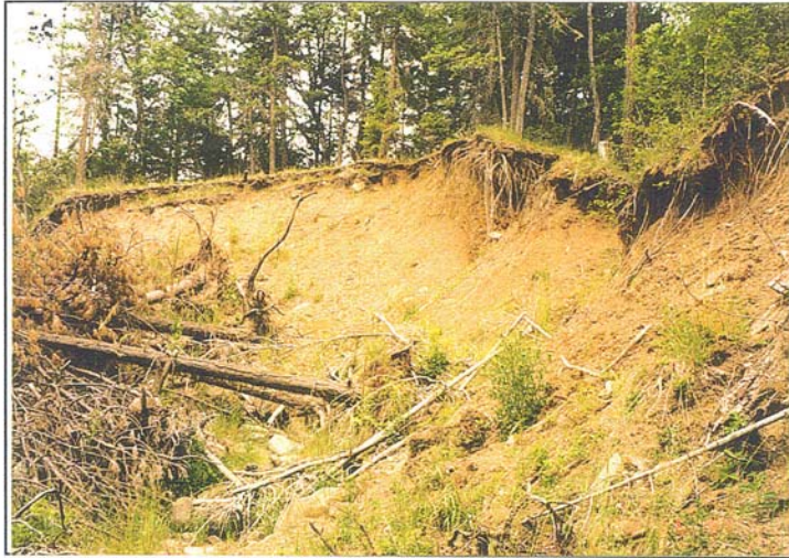
Photograph No. 8. Tyler Creek Wasteway. Looking upstream from Station 64+40 at 30-foot high erosional wall of channel. Numerous toppled trees are to the left and undercut trees are to the right. USBR Photograph by B.H. Carter, 6/26/97.
