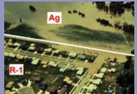
A land use plan or zoning ordinance should designate flood-prone lands for agricultural, conservation, or other uses that suffer minimal damage from a flood.
