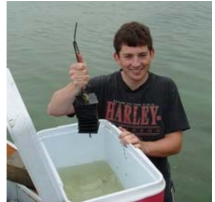
Undergraduate Student Ross Vander Vorste with Hester-Dendy Sampler used for invertebrate collection.
