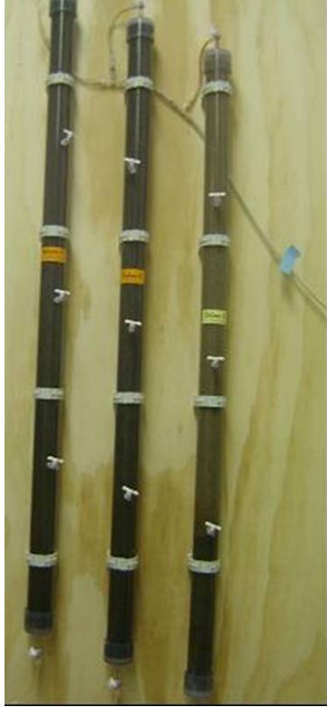
Figure 5. Photograph of continuous flow columns in the laboratory to test the effectiveness and longevity of chitin for the remediation of acid mine drainage.
