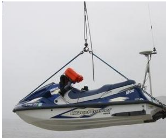
Figure 2. The WaveRunner survey system is capable of measuring water depths from approximately 0.4 m to 15 m.
