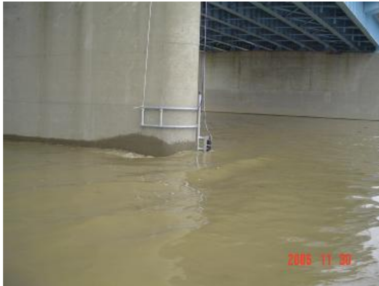
Figure 4. Snapshot of an IMAGENEX deployment at the proposed Hamilton site (ODOT ID-BUT-128-0855). Figure courtesy of Dave Straub (USGS).
