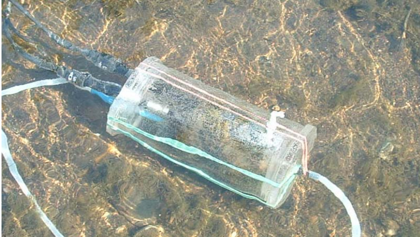
Figure 1: Second-generation flux-chamber, fitted with WTW Multi-340i.
