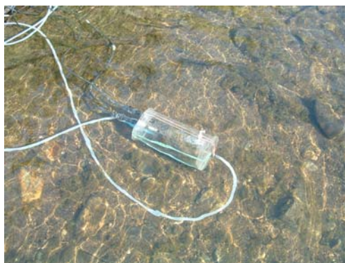
Figure 3: One of the isolation (flux) chambers used in the BHR. Tubing is connected to a streamside peristaltic pump. Conductivity, dissolved oxygen and pH probes are inserted into the chamber and it is filled with small rocks and periphyton.
