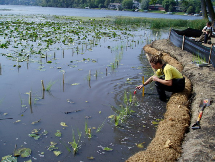
Figure 1. Planting Scirpus validus at Lake Sweeney, Hennepin County. Each plant received a unique identification number. The position of each plant was randomized and its location within the plot was recorded on the wooden lathe stakes and on a master plan so that each plant's mortality can be tracked.
