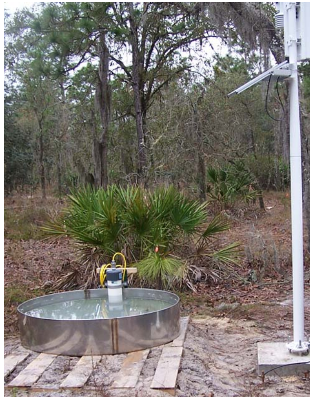
Figure 6. Class A ET pan with GeoKon water level monitoring device installed next to the weather station.
