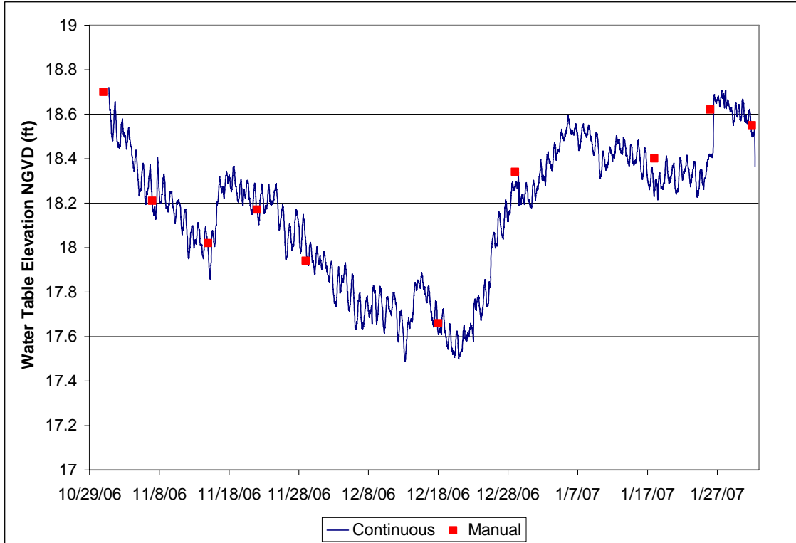
Figure 29. Continuous water-table measurements at FL-02 with weekly manual measurements.
