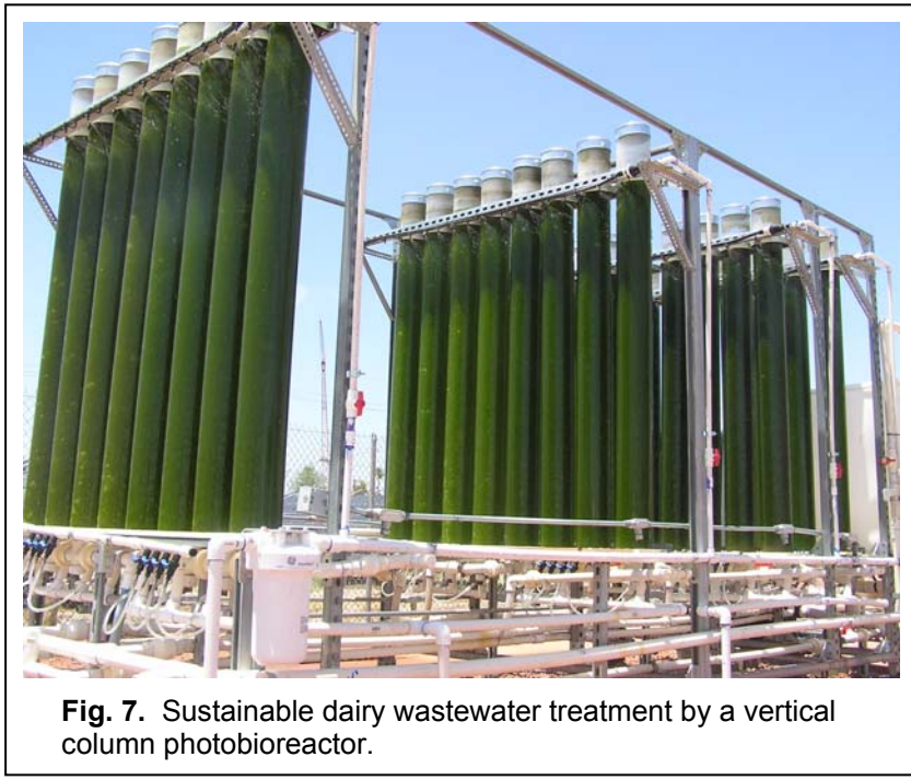
Fig. 7 demonstrates the technical feasibility of ammonia removal from dairy wastewater using the vertical column photobioreactor outdoors. Quantitative assessment of the vertical column reactor for dairy wastewater bioremediation is underway.
