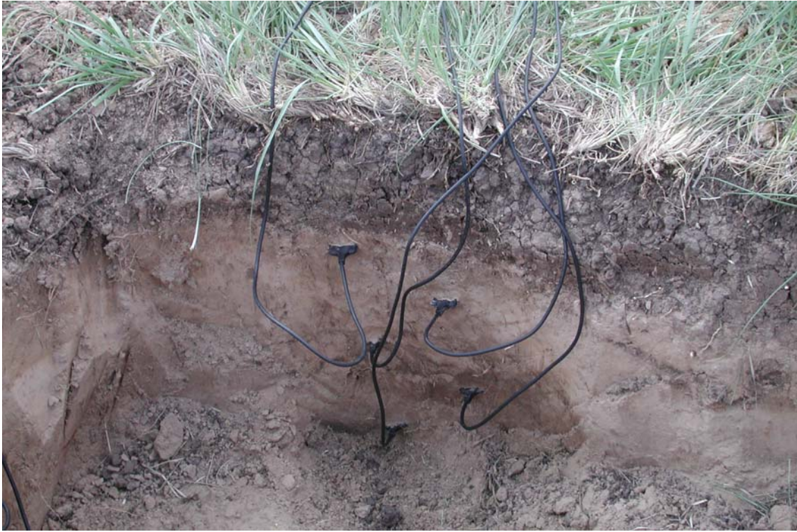
Figure 2 – Pit Ash22 with installed sensors
